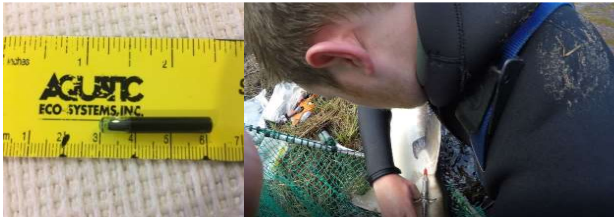
Left: 23 mm Radio Frequency Identification Tag (RFID). Right: Technician Zack Witzel implanting an RFID tag into an adult Lake Sturgeon.
